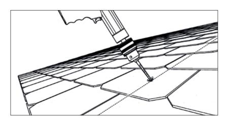
While the roof covering is pre-drilled with Ø 15mm, the substructure must also be predrilled with Ø 7mm for M10 hanger bolts and with Ø 8.5mm for M12 hanger bolts. When pre-drilling into wooden substructures, please make sure that a 90° angle is maintained. Please remove all splinters and cuttings prior to continuing with the work.
