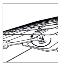
The pre-assembled hanger bolt seal is pressed into the drill-hole of the nub. The conical end of the seal must be fully inserted. The flange nut is then tightened until it sits flush with the sealing ring. Now turn the flange nut the corresponding number of times to compress the seal.
