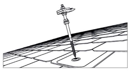
Please observe the minimum specified thread engagement when placing the hanger bolts. For M10 hanger bolts, this minimum thread engagement is 60mm and for M12 hanger bolts it is 100mm. You will need a size 7 socket for M10 hanger bolts and a size 9 socket for M12 hanger bolts.
