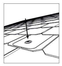
Insert Slide SlatePlan along the axis between the shingles. Now mark the penetration points for the hanger bolts. The SlatePlan must now be removed before carrying out the next steps.
