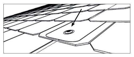
Reinsert the SlatePlan and arrange the drill holes exactly one above the other.
