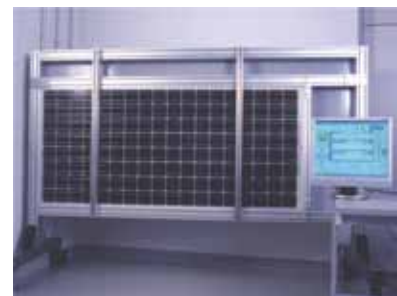
Example of a module loading test in an overpressure/underpressure test set-up (VDE)
