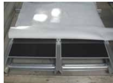
Example of a module loading test with water bag (Schletter) (Preparation of the test set-up)
