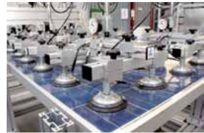
Example of a module loading test with vacuum suction (TÜV Rheinland)
